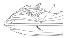
1 Cooling water pilot outlet (port [left] side)
