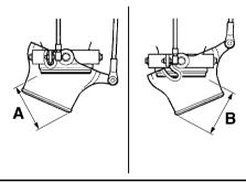
Difference between fully turned positions of jet thrust nozzle (distances A and B):
