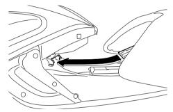
(2) Push the rear of the seat down to securely lock it in place.
