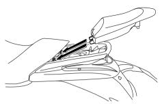
(2) Push the rear of the seat down to securely lock it in place.
