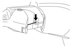
Steering cable (jet thrust nozzle end) and Q.S.T.S. rod (jet thrust nozzle end)
