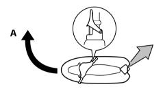
B. Less throttle produces lower thrust, so the watercraft will turn more gradually.
