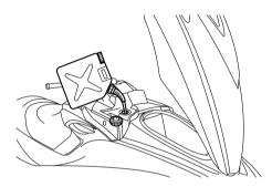
(7) Stop filling when the fuel level reaches approximately 50 mm (2 in) from the top of the fuel tank. Do not overfill the fuel tank. Because fuel expands when it heats up, heat from the engine or the sun can cause fuel to spill out of the fuel tank. Do not leave the watercraft with a full tank in direct sunlight.
