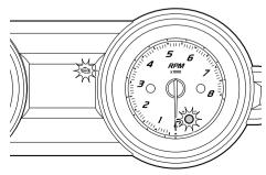
If the check engine warning is activated, immediately reduce the engine speed, return to shore, and have a Yamaha dealer check the engine.
