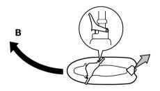
C. Releasing the throttle lever completely produces only minimum thrust. If you are traveling at speeds above trolling, you will have rapidly decreasing ability to steer without throttle. You may still have some turning ability immediately after releasing the throttle lever, but once the engine
