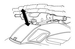
(2) Make sure that the lock lever returns to its original position and that the handlebars are securely locked in place.
