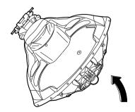
(2) Remove any weeds or debris from around the jet intake, drive shaft, impeller, jet pump housing, and jet thrust nozzle.
