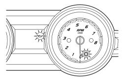
If the oil pressure warning is activated, immediately reduce the engine speed, return to shore, and then check the engine oil level. (See page 51 for information on checking the engine oil level.) If the oil level is sufficient, have a Yamaha dealer check the watercraft.
