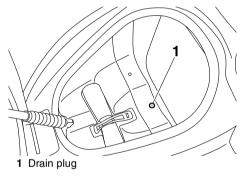
Securely install the drain plug in its original position.
