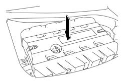
(2) Install the engine cover screws, and then tighten them to the specified torque.
