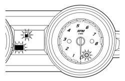
If the fuel level warning is activated, refill the fuel tank as soon as possible. (See page 49 for information on filling the fuel tank.)
