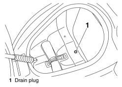
(2) Securely install the drain plug in its original position.
