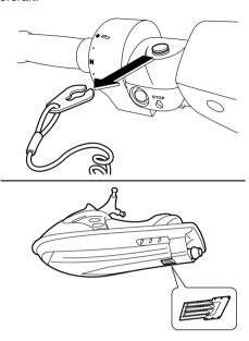
(1) Place a suitable clean cloth or carpeting underneath the watercraft to protect it from abrasions and scratches. Turn the watercraft on its side as shown. NOTICE: Always turn the watercraft over onto its port (left) side. When turning the watercraft on its side, support the bow so that the handlebars are not bent or damaged. [ECJOOS61]
