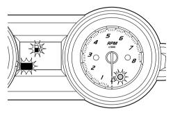
If the fuel level warning is activated, refill the fuel tank as soon as possible. (See page 49 for information on filling the fuel tank.)
