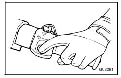
Attach the clip ① to the engine shut-off switch ② and attach the engine shut-off cord ③ to your left wrist.
