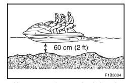
Never operate in water that is less than 60 cm (2 ft) deep, otherwise you increase your chance of hitting a submerged object, which could result in injury.
