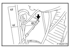
• Steering cable (handlebar end)
