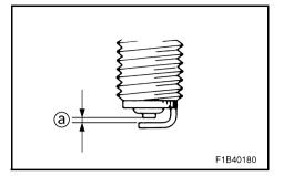
Measure the spark plug gap ⓐ with a wire thickness gauge. Replace the spark plug or adjust the gap to specification if necessary.
