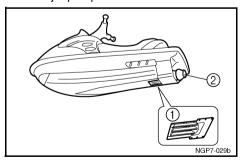
Stop the engine and remove the clip ③
