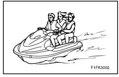
This watercraft is designed to carry the operator and up to 2 passengers. Never exceed the maximum load limit or allow more than 3 persons (or 2 persons if a water-skier is being pulled) to ride the watercraft at one time.
