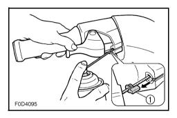
Throttle cable (handlebar end)
