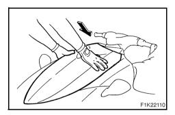
To close the hood, push the hood down to lock it in place.
