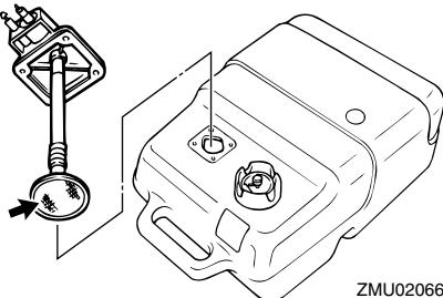
4. Clean the filter (located on the end of the suction pipe) in a suitable cleaning solvent. Allow the filter to dry.
