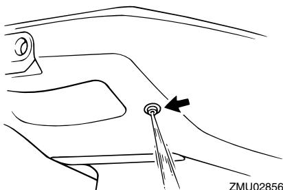
Check that no water leaks from the joints between the exhaust cover, cylinder head, and body cylinder.
