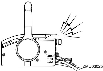
If the alert system has been activated, stop the engine and check for the cause.
