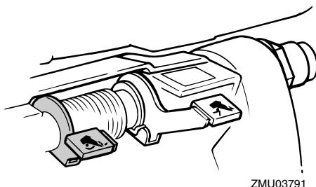
3. To set the outboard motor in a partially tilted position, slightly tilt the outboard motor up until the plate turns completely.
