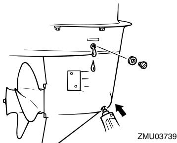
6. Put a new gasket on the oil level plug. When the oil begins to flow out of the oil level plug hole, insert and tighten the oil level plug.
