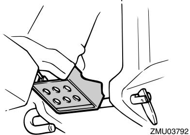
4. To return the outboard motor to the normal running position, place the remote control lever / gear shift lever in neutral, then slightly tilt the outboard motor up. Set the tilt lock lever and shallow water lever to the lock position and slowly tilt the outboard motor down.
