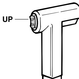
3. To return the outboard motor to the normal running position, press the power trim and tilt switch and slowly tilt the outboard motor down.
