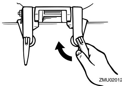
2. If the engine restraint cable attachment is equipped on your engine, an engine restraint cable or chain should be used. Attach one end to the engine restraint cable attachment and the other to a secure mounting point on the boat. Otherwise the engine could be completely lost if it accidentally falls off the transom.
