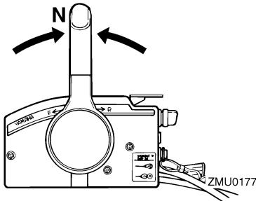
2. Slightly tilt the outboard motor up to the desired position using the power trim and tilt switch. **WARNING! Using the power trim and tilt switch on the bottom cowling while the boat is moving or engine is on could increase the risk of falling overboard and could distract the operator, increasing the risk of collision with another boat or an obstacle.** [EWM01850]
