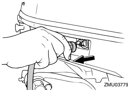
3. Tighten the air vent screw on the fuel tank cap (if equipped).
