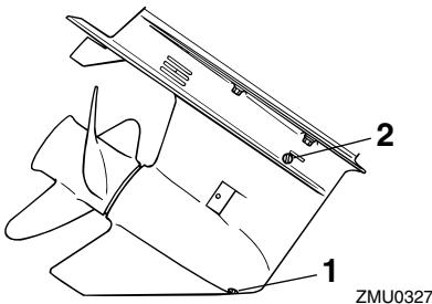
1. Gear oil drain screw
