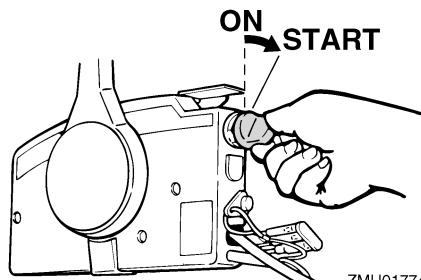
5. Immediately after the engine starts, release the main switch and allow it to return to “ON” (on).
