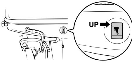
3. Press the power trim and tilt switch / power tilt switch "UP" (up) until the outboard motor has tilted up completely.
