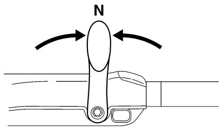
2. Pull the tilt lock lever up to the release position.
