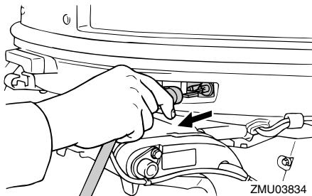
3. Tighten the air vent screw on the fuel tank cap (if equipped).
