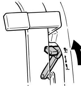
3. Slightly tilt the outboard motor up to the desired position and push the tilt lock lever down to the lock position.
