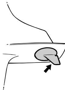
4. Clean the filter (located on the end of the suction pipe) in a suitable cleaning solvent. Allow the filter to dry.
