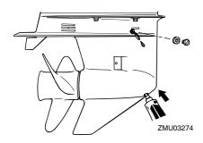
Put a new gasket on the oil level plug. When the oil begins to flow out of the oil level plug hole, insert and tighten the oil level plug.
