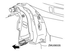
Make test runs with the trim set to different angles to find the position that works best for
