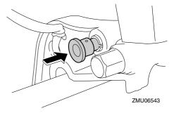
4. Models equipped with trim rods: Once the outboard motor is supported with the tilt support lever, press the power trim and tilt switch "DN" (down) to retract the trim rods. NOTICE: Make sure that the trim rods retracts completely during mooring. This protects the rods from marine growth and corrosion, which could damage the power trim and tilt mechanism. [ECM00252]
