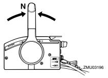
Press the power trim and tilt switch "UP" (up) until the outboard motor has tilted up completely.
