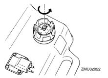
If there is a fuel joint on the motor, align the fuel joint on the fuel line with the fuel joint on the motor and firmly connect the fuel line to the joint while pinching the joint. Then firmly connect the other end of the fuel line to the joint on the fuel tank.
