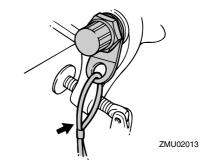
Secure the clamp bracket to the transom using the bolts provided with the outboard (if packed). For details, consult your Yamaha dealer. WARNING! Avoid using bolts, nuts or washers other than those contained in the engine packaging. If used, they must be of at least the same quality of material and strength and must be tightened securely. After tightening, test run the engine and check their tightness.
