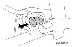
Push the power trim and tilt switch "DN" (down) to lower the outboard motor to the desired position.
