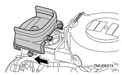
Remove the grommet and disconnect the start-in-gear protection cable from the manual starter.
