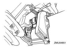
4. To return the outboard motor to the normal running position, place the remote control lever / gear shift lever in neutral.
