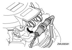
Remove the flywheel magnet cover after removing the bolt(s).
