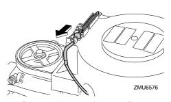
Remove the manual starter after removing the bolt(s).
