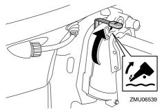
Slightly tilt the outboard motor up. The tilt support bar will lock automatically, supporting the outboard motor in a partially raised position. This outboard motor has 2 positions for shallow water cruising.
