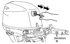
After the engine starts, slowly return the manual starter handle to its original position before releasing it.
