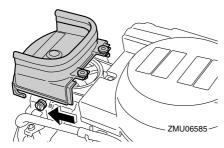
Pull off the 10-pin connector from the clamp and remove the flywheel magnet cover (if equipped).
