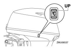
To return the outboard motor to the normal running position, press the power trim and tilt switch and slowly tilt the outboard motor down.
