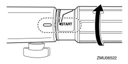
Pull the manual starter handle slowly until you feel resistance. Then give a strong pull straight out to crank and start the engine. Repeat if necessary.
