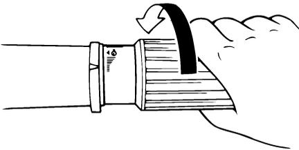
2. After the engine is at idle speed in gear move the gear shift lever firmly and crisply into the neutral position.
