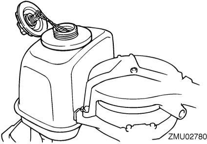
1. With the outboard motor tilted down (in the vertical running position), remove the fuel tank cap.
