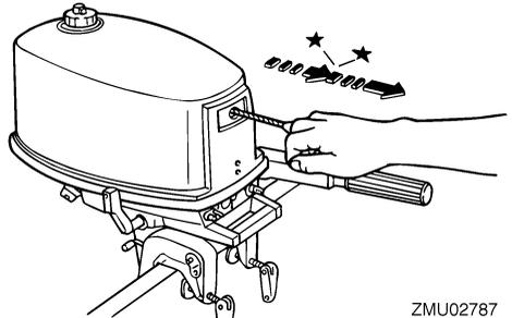
6. After the engine starts, slowly return the manual starter handle to its original position before releasing it.
