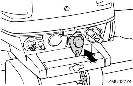
2. After stopping the engine, tighten the air vent screw on the fuel tank cap and set the fuel cock lever or knob to the closed position, if equipped.
