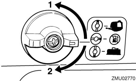
1. "OPEN" position for the built-in tank
