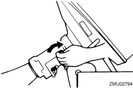
3. If equipped with the tilt support knob: Pull the knob out, and then slowly tilt the outboard motor down.
