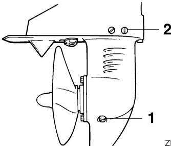
1. Gear oil drain screw
