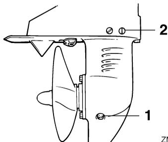
1. Gear oil drain screw
