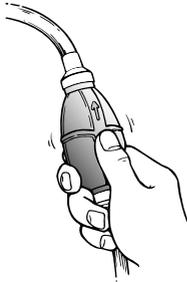
4. Open the throttle slightly without shifting using the throttle grip, neutral throttle lever or free accelerator. It is necessary to change the throttle opening slightly depending on the engine temperature. After the engine starts, return the throttle to its original position.
