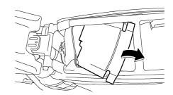
Remove the air filter element by removing the wing bolt and its washer.
