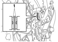
1. Brake pad wear indicator groove
