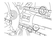
The pivoting points of the rear suspension must be lubricated by a Yamaha dealer at the intervals specified in the periodic maintenance and lubrication chart.
