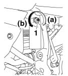
1. Compression damping force adjusting screw
