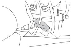
Remove the spark plug as shown, with the spark plug wrench included in the owner's tool kit.
