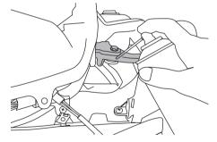
The pivoting points of the front and rear brake levers must be lubricated at the intervals specified in the periodic maintenance and lubrication chart.
