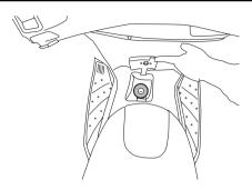
Insert the key into the lock and turn it 1/4 turn counterclockwise. The lock will be released and the fuel tank cap can be removed.
