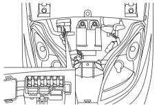
The main fuse and the fuse box, which contains the fuses for the individual circuits, are located behind cowling B. (See page 6-5.)
