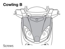
Remove the screws, and then take the cowling off.
