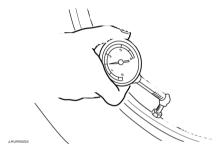
The tire air pressure should be checked and, if necessary, adjusted before each ride.
