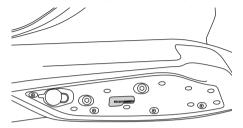
The vehicle identification number is stamped into the frame.
