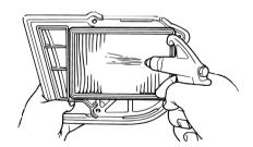
2. Remove the air filter element, and then blow out the dirt with compressed air as shown.
