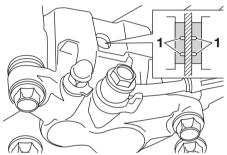
The rear brake is provided with a check plug, which, if it is removed, allows you to check the brake pad wear without disassembling the brake. To check the brake pad wear, check the position of the wear indicator while applying the brake. If a brake pad has worn to the point that the
