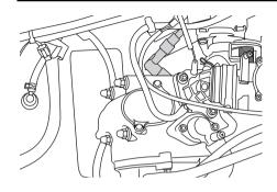
3. Remove the spark plug cap.
