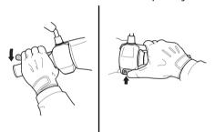
3. Start the engine by pushing the start switch while applying the front or rear brake.
