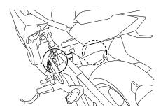
The swingarm pivots must be lubricated by a Yamaha dealer at the intervals specified in the periodic maintenance and lubrication chart.
