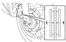
1. Brake pad wear indicator groove
