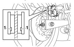
1. Brake pad wear indicator groove
