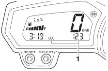
1. Odometer/tripmeter/fuel reserve tripmeter
