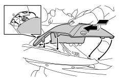
2. Install the bolt and the quick fastener.
