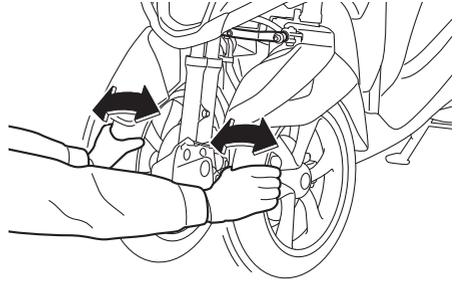
The steering tie rod must be checked at the intervals specified in the periodic maintenance and lubrication chart. If there is play in the steering tie rod, have a Yamaha dealer check the tie rod.
