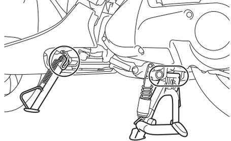
The operation of the centerstand and sidestand should be checked before each ride, and the pivots and metal-to-metal contact surfaces should be lubricated if necessary.
