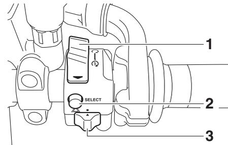
1. Motorstart-/stopptaster “ $\text{M} / \text{O} / \text{X}$ ”
