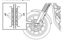
1. Brake pad wear indicator groove
