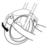
The front and rear wheel bearings must be checked at the intervals specified in the periodic maintenance and lubrication chart. If there is play in the wheel hub or if the wheel does not turn smoothly, have a Yamaha dealer check the wheel bearings.
