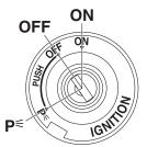
The main switch controls the ignition and lighting systems. The various main switch positions are described below.
