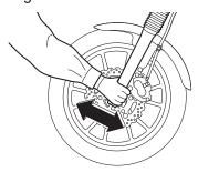
Checking the wheel bearings
