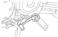
Recommended lubricant: Lithium-soap-based grease Checking and lubricating the brake and clutch levers
