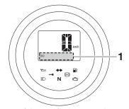
Odometer/tripmeter/fuel reserve tripmeter/clock
