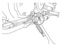
The operation of the sidestand should be checked before each ride, and the sidestand pivot and metal-to-metal contact surfaces should be lubricated if necessary.
