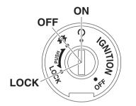
The main switch/steering lock controls the ignition and lighting systems, and is used to lock the steering. The various positions are described below.
