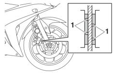
1. Brake pad wear indicator groove
