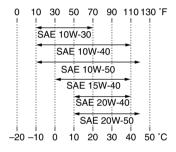
Recommended engine oil grade: API service SG type or higher, JASO standard MA Engine oil quantity: Without oil filter cartridge replacement: 1.80 L (1.90 US qt, 1.58 Imp.qt) With oil filter cartridge replacement: 2.10 L (2.22 US qt, 1.85 Imp.qt) Coolant quantity: Coolant reservoir (up to the maximum layer
