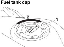
1. Fuel tank cap lock cover 2. Unlock
