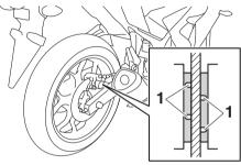
1. Brake pad wear indicator groove
