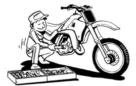
3. During disassembly, check and measure the required parts, and make a record of them so that you may refer to the record when installing them. Moreover, arrange gears, cylinders, pistons, and other parts for each section so as not to confuse or lose them.
