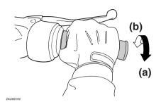
The speed can be adjusted by opening and closing the throttle. To increase the speed, turn the throttle grip in direction (a). To reduce the speed, turn the throttle grip in direction (b).
