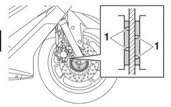
1. Brake pad wear indicator groove
