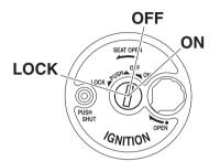
The main switch/steering lock controls the ignition and lighting systems, and is used to lock the steering. The various main switch positions are described below.
