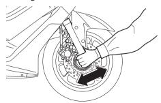
Checking the wheel bearings
