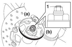
Compression damping force adjusting bolt (for slow compression damping)
