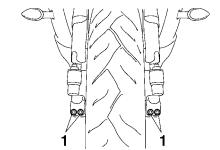
1. Front wheel axle pinch bolt
