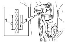
1. Brake pad wear indicator groove
