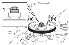
1. Spring preload adjusting bolt
