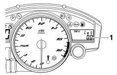
1. Odometer/tripmeter/fuel reserve tripmeter/stopwatch
