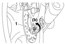
1. Drive chain slack adjusting bolt
