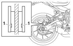
1. Brake pad wear indicator groove
