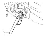
The operation of the sidestand should be checked before each ride, and the sidestand pivot and metal-to-metal contact surfaces should be lubricated if necessary.
