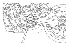
The swingarm pivots must be lubricated by a Yamaha dealer at the intervals specified in the periodic maintenance and lubrication chart.
