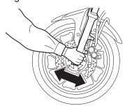
Checking the wheel bearings
