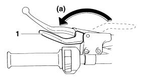
1. Parking brake lever (locked position)
