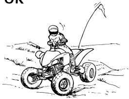
If your ATV has stalled or stopped and you believe you can continue up the hill, restart carefully to make sure you do not lift the front wheels which could cause you to lose control. If you are unable to continue up the hill, dismount the ATV on the uphill side. Physically turn the ATV around and then descend the hill.
