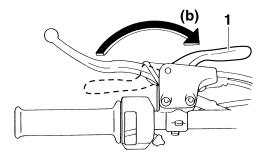
1. Parking brake lever (unlocked position)
